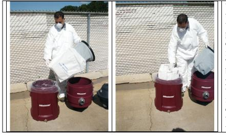
7. When you are through using the vacuum, remove the pre-filter from the cloth filter and put it into the plastic liner. This pre-filter should be changed every time you empty the vacuum. The pink impact filter should be changed every other time you empty the vacuum.
