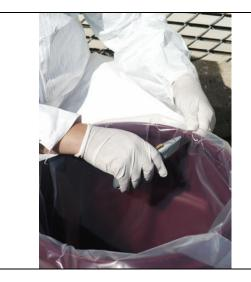
2. Next, cut a 1" slit in the plastic recovery bag at the top of the tank directly across from the intake. This will prevent the vacuum from trying to suck the bag up into the vacuum motor.
