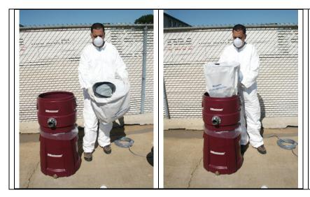
4. Next, gently slide the filter protector (part # 805038pkg) over the cloth filter. Place the cloth filter with the filter protector into the uniadaptor. 5. Next attach the pink impact filter (part # 110005pkg) to the H.E.P.A. filter which is mounted on the bottom of the lid assembly. Line up the black tabs on the impact filter with the raised notches on the H.E.P.A filter and push into place.
