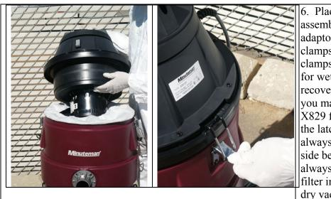
6. Place the lid assembly onto the uniadaptor and fasten the 2 clamps. Note the clamps have 2 positions for wet recovery or dry recovery. Even though you may be using the X829 for wet recovery, the latches should always go onto the dry side because you will always be using a bag filter in the X829 wet dry vacuum.
